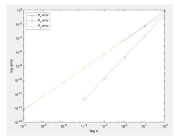
This plot is much more readable! It shows us that  $P_1$  and  $P_3$  have about the same error at  $x \to 0$ , whereas the error in  $P_2$  decreases significantly faster. In fact, the error for  $P_2$  grows so small for small values of x that it is rounded to zero during the calculation, which is why several points are absent from the graph of  $P_2$  (because the log of zero is undefined).
