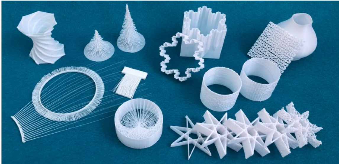
Figure 1: Prints created using the ExtruderTurtle library.
