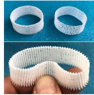
Figure 12: Flexible circles with different extrusion densities, affecting their flexibility and transparency.
