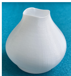
Figure 15: Nonplanar vase with a sinusoidal oscillation along the rim.
