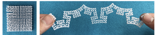
Figure 6: A 3D-printed Hilbert curve relaxed and extended.
